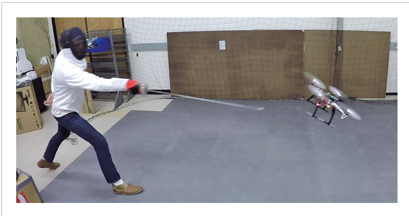
Figure 2. Demonstrating real-time kinodynamic planning on a quadrotor dodging a fencing blade.
