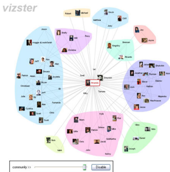
Fig. 6. Vizster interface [28] introduced to visualize network structures based on a force-directed layout algorithm. The colored overlays represent communities identified within the network.
