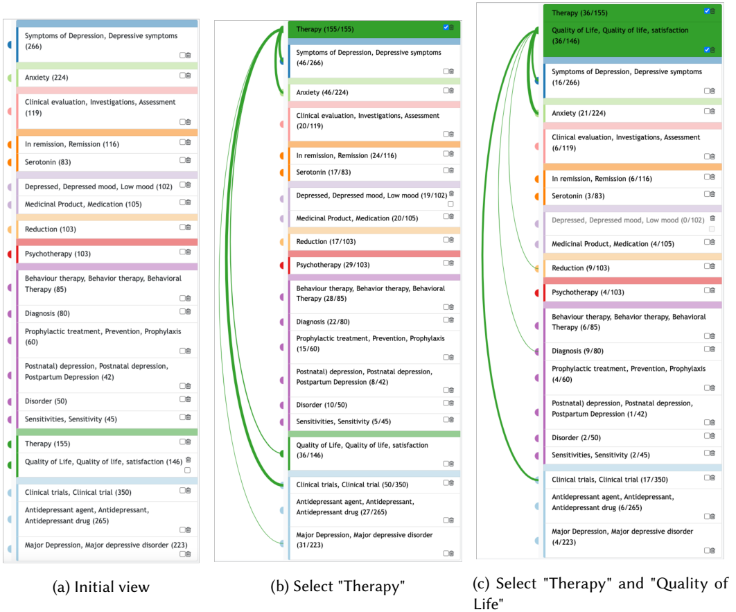
Fig. 5. Facet list transitions. (a) The user starts with an initial view. (b) After the concept “Therapy” is selected, it is moved to the top of the facet list. Arcs are drawn to connect the selected concept to the five most related concepts. The arcs have the same color as the selected concept. (c) A second concept “Quality of Life” is selected, and it is also moved to the top of the facet list. Relations between the intersection of the selected two concepts (at the top) and the other concepts are again shown by arcs.
